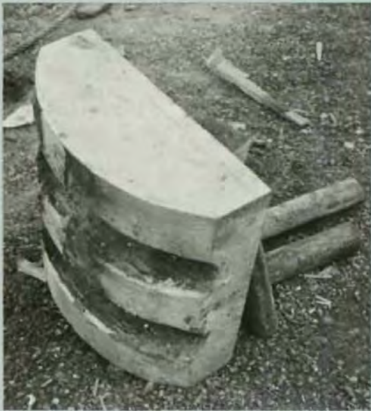
Cast iron cable saddle and roller assembly.
