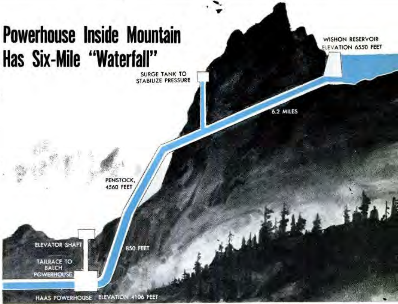
Profile sketch illustrates the flow of water to underground Haas powerhouse from High Sierra reservoir
